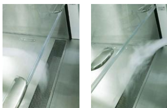
Forms an air barrier from inside and outside of the workspace.
